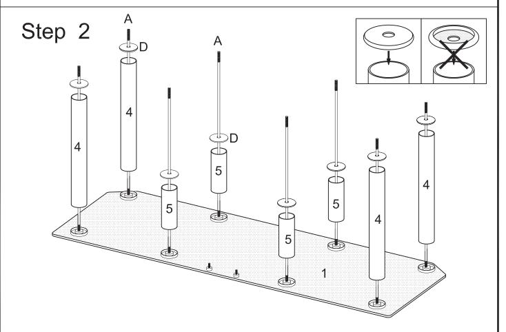
Slide cylinders (4) onto outside long rods (A). Slide cylinders (5) onto middle long rods (A). Slide decorative rings (D) onto long rods (A) and snap onto cylinders (4,5).
